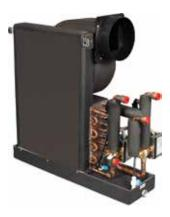
The ATV is a chilled water air handler designed for applications where very little depth is available. In the "4-pipe" configuration there are two separate sets of valves and heat exchangers for cooling and for heating. Two pipes connect to the chiller system to provide cooling, and two pipes connect to an auxiliary heat source, such as a boiler, to provide heating.
