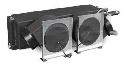
The ABL-HV series of draw-through air handlers for chilled water systems is ideal for installation in height-restrictive spaces. Insulating foam covers the condensate pan, blower housing, shroud, and coil end cover to reduce noise and secondary condensation. The condensate pan also has an antislosh, anti-fungal foam lining. The ABL-HV series is designed to replace the CBLB models.
