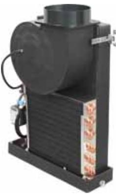
ATV-HV chilled water air handlers were designed for applications where very little depth is available. Showcasing a unique vertical layout, these air handlers have the coil low and the blower above.
