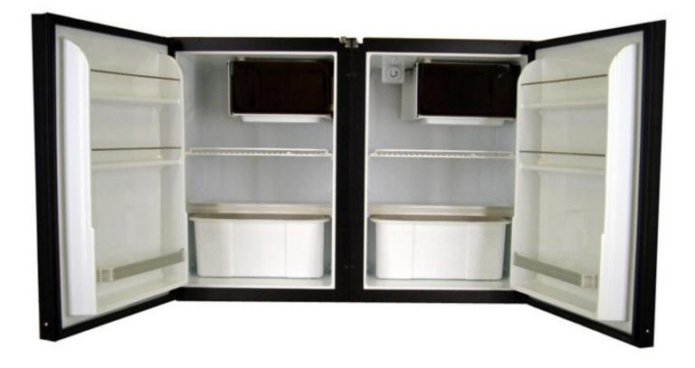
Interior Volume CuFt. 7 Freezer Volume CuFt. 0.8 Voltage: 12/24VDC 110/220VAC Weight Lbs: 93 Cut Out: 28 3/8 H x 41 1/4 W x 18 1/2 D Flange Dimensions: 29 3/8 H x 42 W Running Amperage: 12vdc 4.4A 24vdc 2.2A
