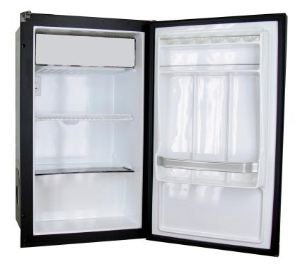
Interior Volume CuFt. 12.1 Freezer Volume CuFt. .25 Voltage: 12/24VDC 110/220VAC Weight Lbs: 45 Cut Out: 28 3/8 H x 16 3/4 W x 14 D Flange Dimension: 29 1/4 H x 17 3/4 W Running Amperage: 12vdc 2.2A 24vdc 1.1A
